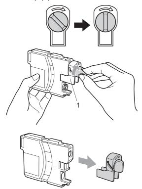
5 Each colour has its own correct position. Insert the ink cartridge in the direction of the arrow on the label.
